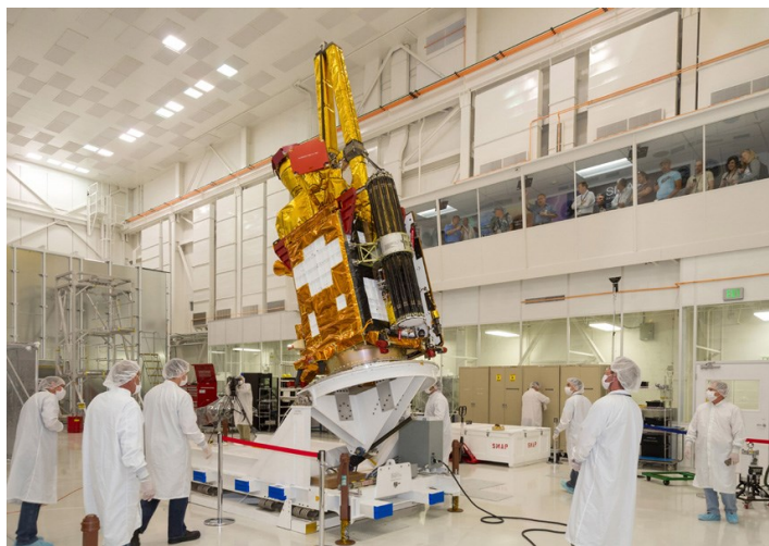
NASA's Soil Moisture Active Passive (SMAP) spacecraft is slowly lowered into place in the Spacecraft Assembly Facility at NASA Jet Propulsion Laboratory, Pasadena, California, in preparation for shipping to California's Vandenberg Air Force Base on October 15.
