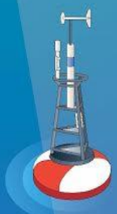
NOAA TAO Array Buoy (Tropical Atmosphere Ocean)
