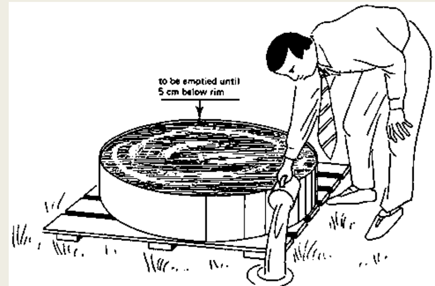
Take water out of the pan when the water depth rises too much
