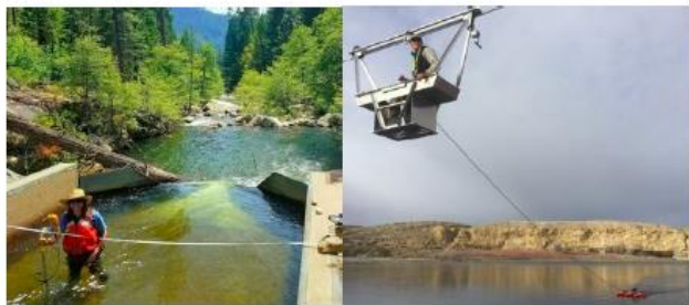
USGS scientists taking velocity and depth measurements
