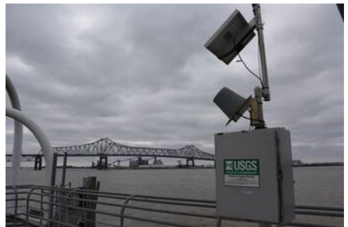
Sources/Usage: Public Domain. A USGS streamgage on the Mississippi River in Baton Rouge, Louisiana.
