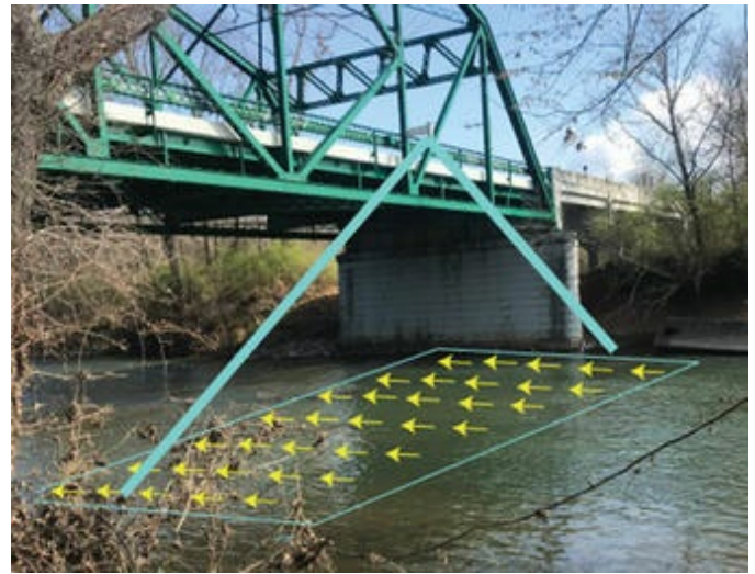
Sources/Usage: Public Domain. The USGS is advancing the use of large-scale particle-image velocimetry (LSPIV), a method that uses innovative video analyzation techniques to measure streamflow.
