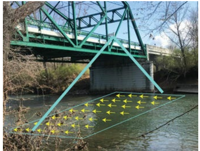
Sources/Usage: Public Domain. The USGS is advancing the use of large-scale particle-image velocimetry (LSPIV), a method that uses innovative video analyzation techniques to measure streamflow.
