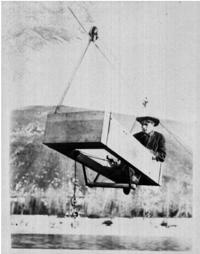
Sources/Usage: Public Domain. A hydrographer taking a cableway streamflow measurement at the first USGS streamgage in Embudo, New Mexico.
