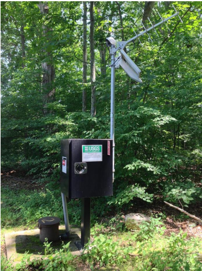
USGS groundwater site 414831072173002 in Tolland County, Connecticut. This well is equipped with a transducer and equipment that allows groundwater level data to be transmitted in real-time.
